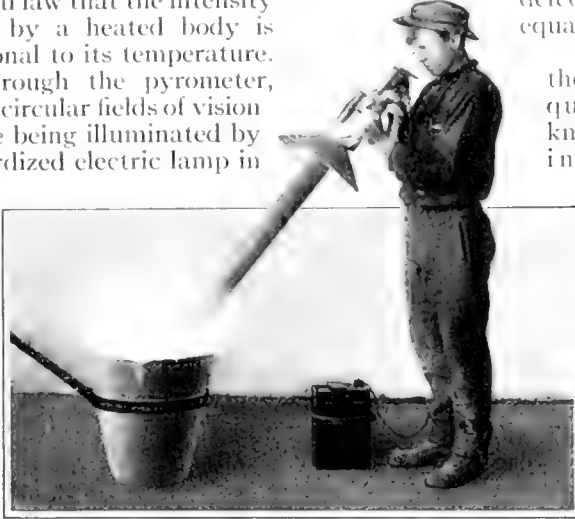
Measuring the White Heat of Molten Minerals. The Shield Protects the Hands of the Operator. The Instrument Also Measures the Heat of Moving Bodies
